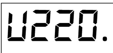
A digital display showing the text 'U220.' in a seven-segment font, indicating the unregulated input voltage.
