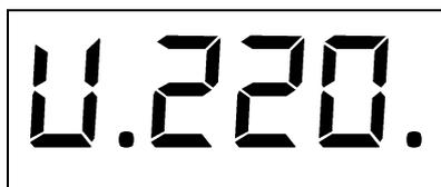
A digital display showing the text 'U.220.' in a seven-segment font, indicating the regulated output voltage.
