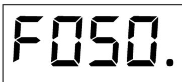
A digital display showing the text F050 with a decimal point at the end, indicating a frequency value of 0.050 Hz.
