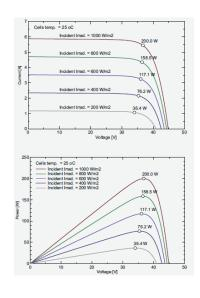
STC: Irradiance 1000W/m $^2$  ,Module temperature 25  $^{\circ}$ C,AM1.5 spectrum.
