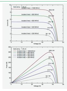
STC: Irradiance 1000W/m² ,Module temperature 25  $^{\circ}\! \mathrm{C}$  ,AM1.5 spectrum.
