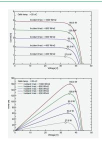
STC: Irradiance 1000W/m  $^2$  ,Module temperature 25  $^\circ\!\!\!\mathrm{C}$  ,AM1.5 spectrum.
