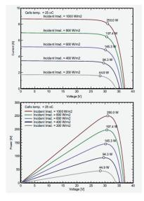
STC: Irradiance 1000W/m² ,Module temperature 25  $^{\circ}\text{C}$  ,AM1.5 spectrum.
