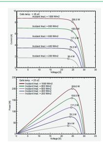
STC: Irradiance 1000W/m $^2$  ,Module temperature 25  $^\circ\!\!\mathrm{C}$  ,AM1.5 spectrum.
