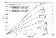
STC: Irradiance 1000W/m² ,Module temperature 25°C ,AM1.5 spectrum.
