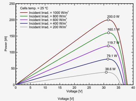
STC: Irradiance 1000W/m<sup>2</sup>, Module temperature 25°C, AM1.5 spectrum.
