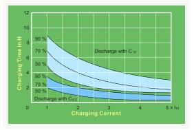
Recharging time in dependence of charging current (guide values) for up to 50, 70 and 90% of capacity at 25°C and with a charging voltage of 2.27 V/cell.
