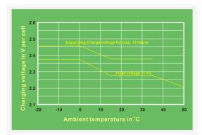
For charging 2.27 V/cell is recommended. The charging voltage must be compensated according to the curve for continuously different battery ambient temperature.
