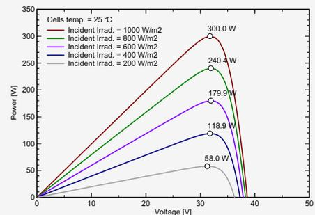
STC: Irradiance 1000W/m<sup>2</sup>, Module temperature 25°C, AM1.5 spectrum.
