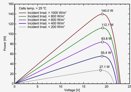
STC: Irradiance 1000W/m<sup>2</sup>, Module temperature 25°C, AM1.5 spectrum.
